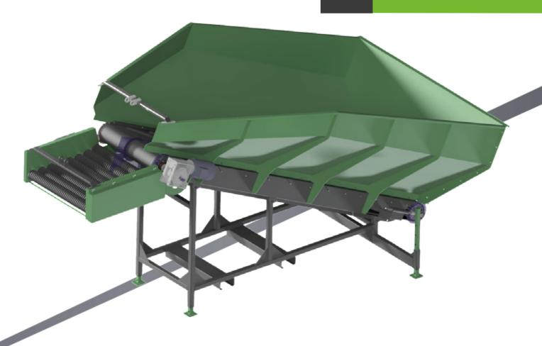
The MACHINES PIÓRO – KS receiving hopper is designed for unloading pallet boxes using a forklift turntable. An appropriately profiled rubber belt allows the vegetables to be transported to the cable-controlled soil separator, which then transfers the goods to the next machine in the vegetable line. Optionally, it can be equipped with an adjustable sorter with a transverse receiving belt \* model S
