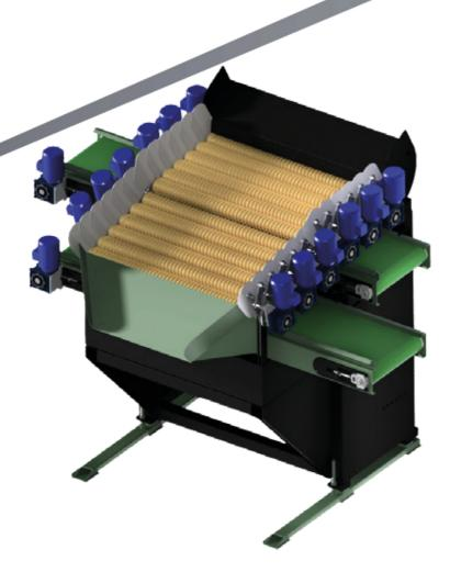
The MACHINES PIÓRO SO100 circulation sorter is used to sort goods with preliminary removal of impurities. The machine is intended for round vegetables (potatoes). Sorting is carried out using a selected perforated belt and appropriately set shakers. During operation, the vegetables fall into the holes in the belt and land on the conveyor transporting the goods to the next stages of processing or to the pallet box.
